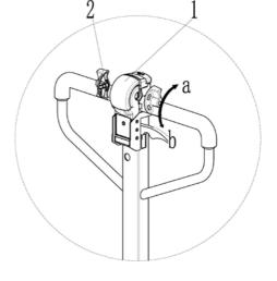
around. When the handle is within the range (B), the brake is close and the truck will stop shortly.
